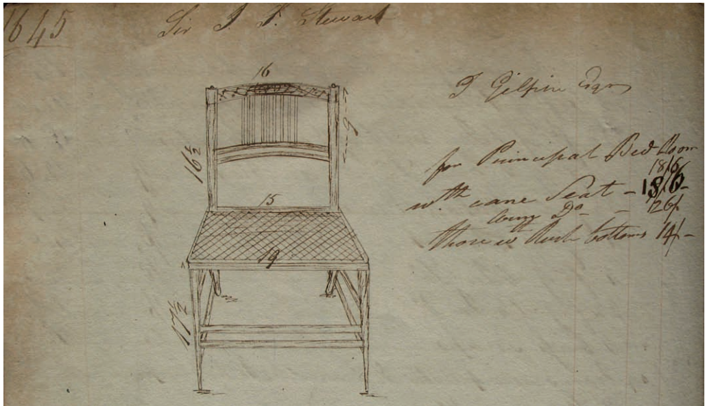
23 Design for Winfred's pattern chair made for Sir John Shaw Stewart of Ardgowan, Renfrewshire in 1801. H 34 in (86.5 cm); w front seat 19 in (48 cm); w back seat 15 in (38 cm). Westminister Archive Centre 344/98, fol. 1645
